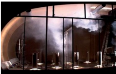
Airflow tests: Mock setup in the TROX research & development laboratory
